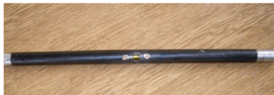
Fig. 7 The shaft model with glued strain gauges
