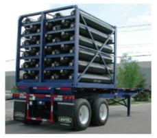
a) ISO 20 ft. container (b) 10 ft. cube for bulk transport *Figure 3: Containers for CNG bulk transport (250 bar modules)*
