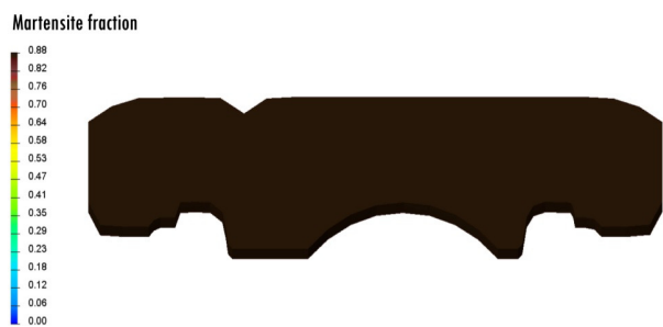
Figure 8. Share of martensite in the bearing ring microstructure after quenching (according to the simulation)
