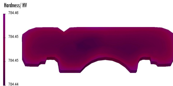
Figure 10. Hardness in the cross section of bearing rings after quenching (according to the simulation)
