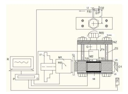
Fig. 1 The scheme of the measurement configuration
