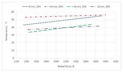
Fig. 5 The influence of radial force on the temperature for various graphite insert diameters and graphite coverages
