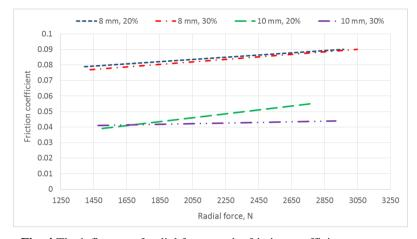
Fig. 4 The influence of radial force on the friction coefficient for various graphite insert diameters and graphite coverage
