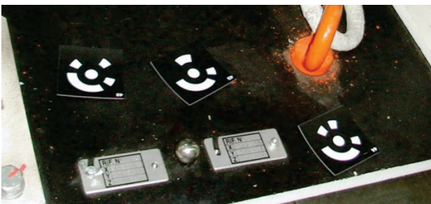
Figure 4 Spheres for transformation of measurement in vehicle coordinate system
