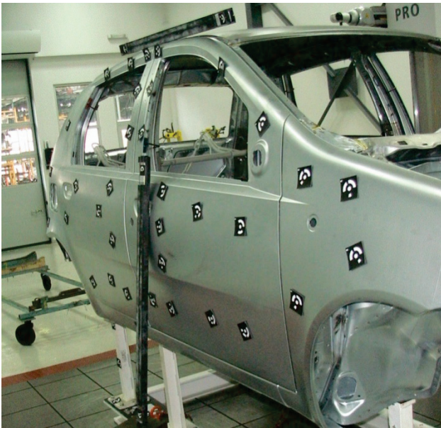
Figure 3 Right side of car prepared for door clearance control
