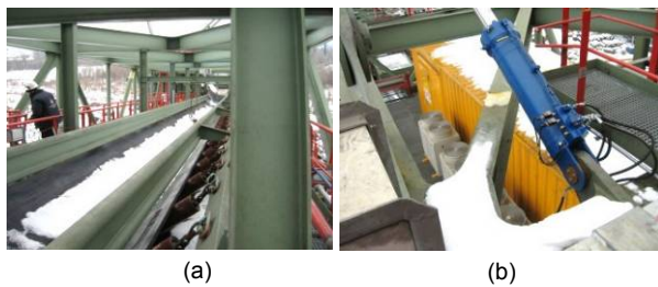
Fig. 14 Level of snow during the second weighing: (a) bucket wheel boom; (b) counterweight boom
