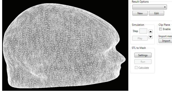
FIGURE 4. Tetrahedral mesh model of head.
