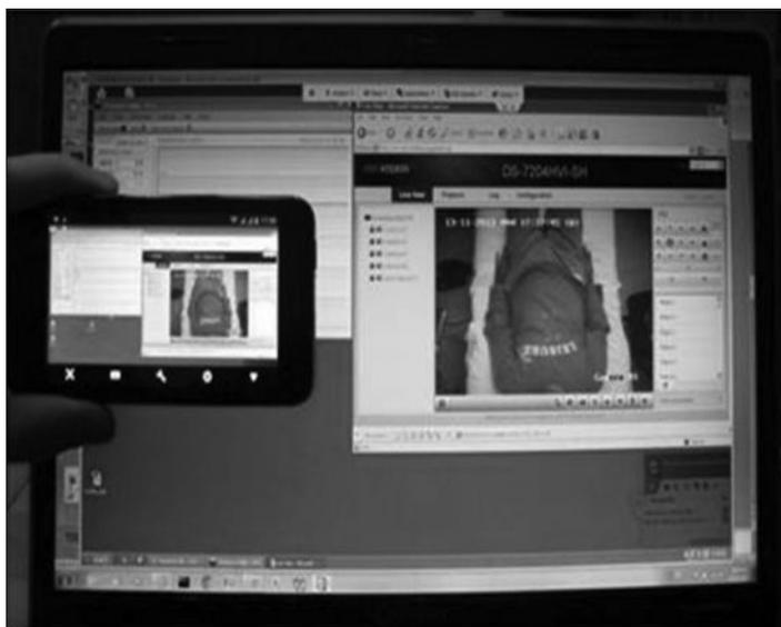
**Fig. 3.** Remote connection to the acquisition computer established with a notebook computer and a smartphone at the physician’s home.
