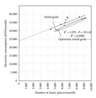
FIGURE 6: Identifying base (target) line.
