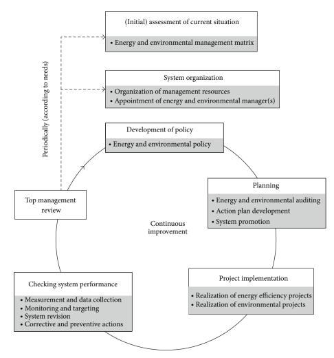
FIGURE 1: Structure of energy and environmental management system (EEMS).
