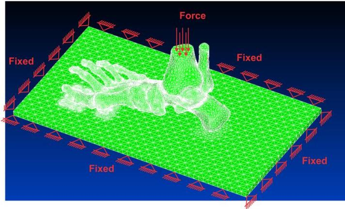
**Fig 4.** Loading of 400 N and fixed boundary condition
