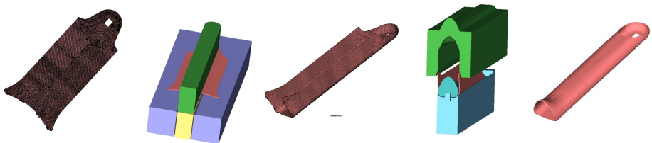
Fig. 6. Numerical models for FE analysis of virtual manufacturing
