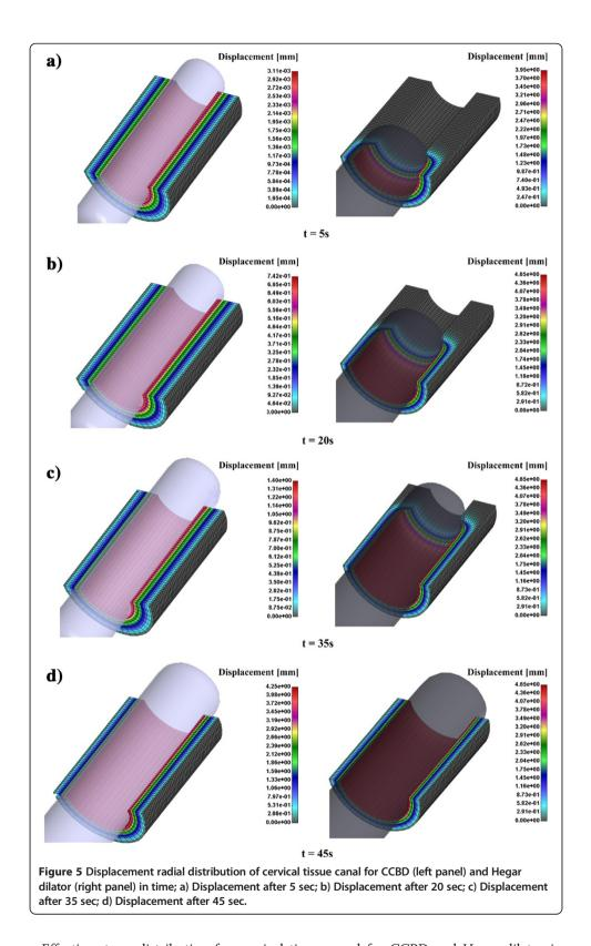
CCBD produces 1.0 kPa which is almost nine times lower. At the end of the dilation process within time frame of 45 sec the effective stress becomes similar in both dilators, which is reasonable because of the similar diameter at that time point.
