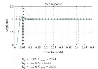
FIGURE 12: System response at the defined damping coefficient  $\xi=0.6$  and the required settling time.
