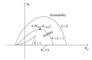
FIGURE 3: Parameter plane with the stability limit.
