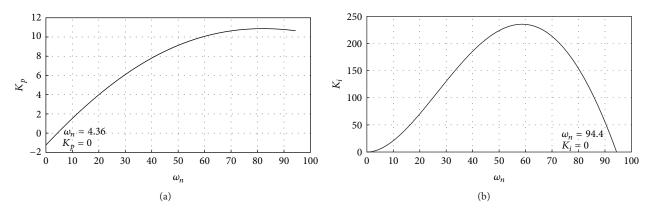
FIGURE 10: Boundary values of the undamped frequency  $\omega_{n \min}$  and  $\omega_{n \max}$  for the damping coefficient of the closed loop  $\xi = 0.6$ .
