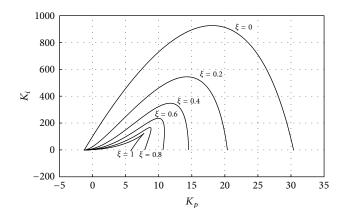
FIGURE 7: Parameter plane for different values of the damping coefficient with the stability limits.
