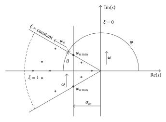
FIGURE 2: Area with the required settling time and relative stability.
