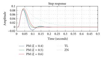
FIGURE 14: Comparative presentation of the system response to the action of load disturbance D=1, for the proposed method (PM), the Ziegler-Nichols method (ZN) and the Tyreus-Luyben method (TL).
