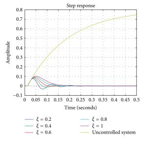
FIGURE 9: Response of the system to the action of disturbance D=1 at  $K_{i\max}$ , for changes of the damping coefficient  $0.2 \le \xi \le 1$ .
