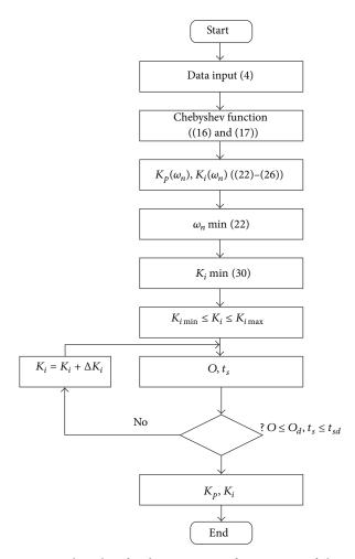
FIGURE 6: Algorithm for determination of parameters of the PI controller.
