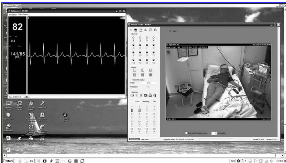
Fig. 3. Live video from surveillance camera and signals from the Nihon Kohden model BSM-2351 Bedside Patient Monitor on one of the desktop computers in the DNM (using the VNC connection on 1 Gbps LAN).
