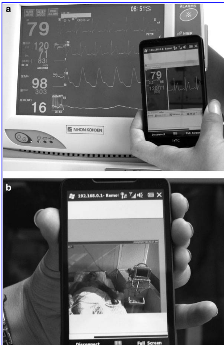
Fig. 5. (a) Signals from the Nihon Kohden BSM-2351 Bedside Patient Monitor on the HTC HD2 mobile phone (using VPN and RDC connections). (b) Live video from the surveillance camera on the HTC HD2 mobile phone (using VPN and RDC connections).
