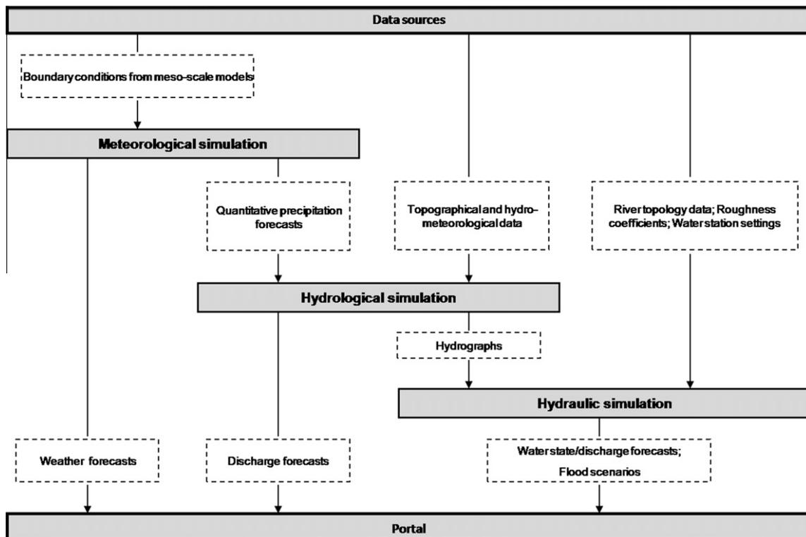
Fig. 1. Workflow of the cascade of simulations for flood forecasting.
