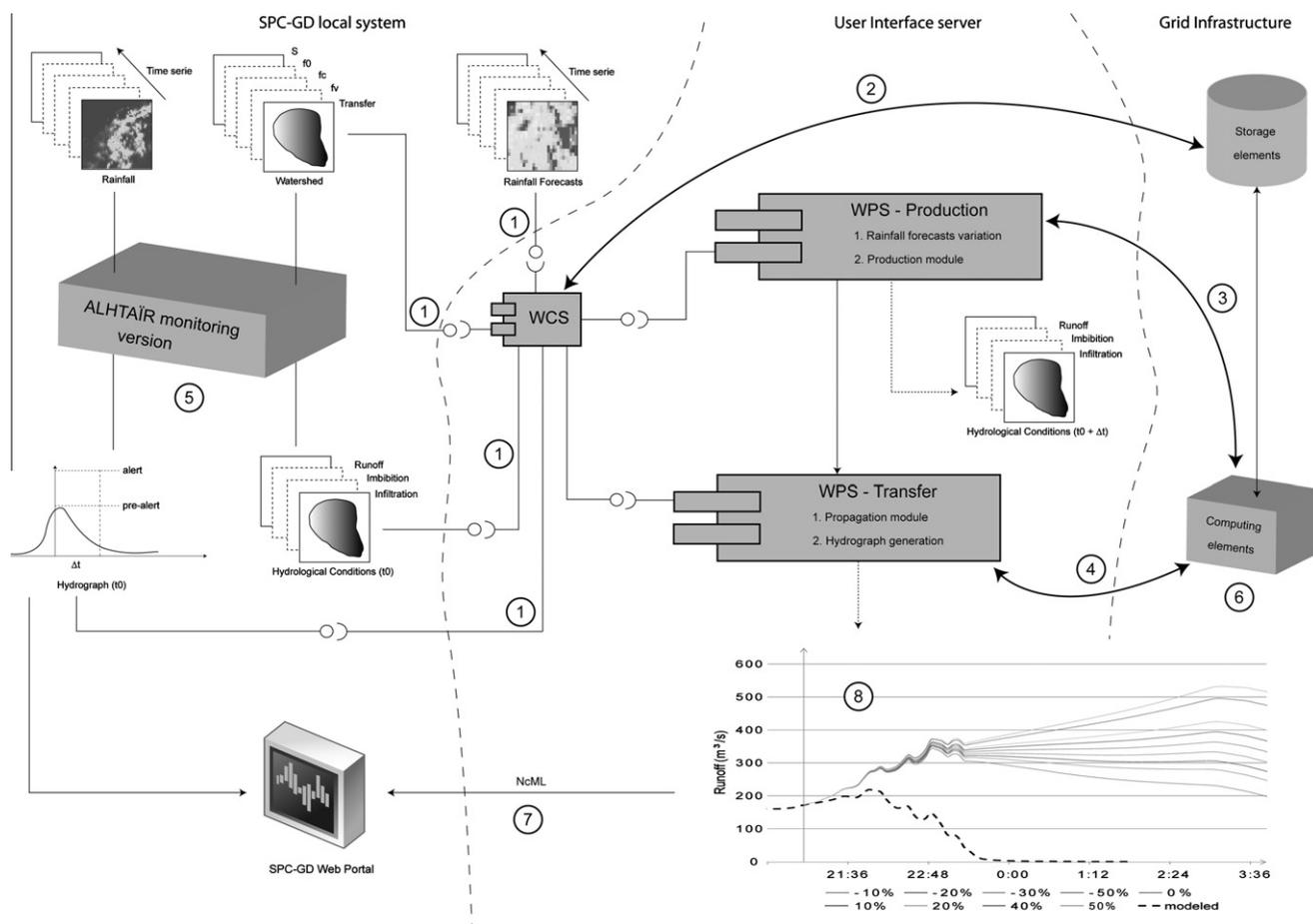
Fig. 3. G-ALHTAIR platform is based on three layers: existing client–server SPC-GD local system, OWS services implemented on the User Interface server and the Grid Infrastructure providing computational and storage resources.
