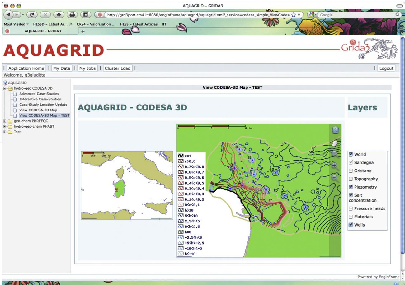
Fig. 4. Piezometric and concentration maps of the seawater intrusion simulation of the Oristano coastal aquifer (Sardinia, Italy) are calculated and displayed on the AQUAGRID computational portal.
