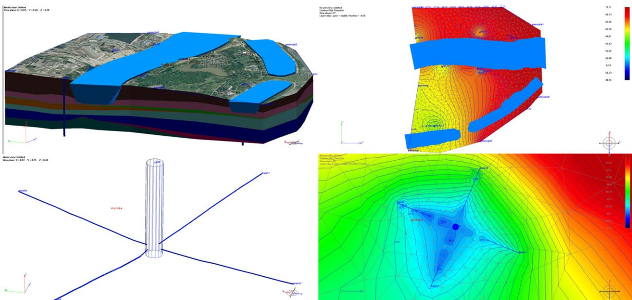
Fig. 5. Topology view of the Belgrade Water Supply Center (top left), single Ranney well with four drains (down left), regional model results – potentials with streamlines (top right) and local model results around the well – potential plot (down right).
