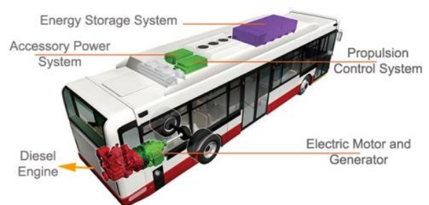
Fig. 2. City bus with integrated hybrid drive system
